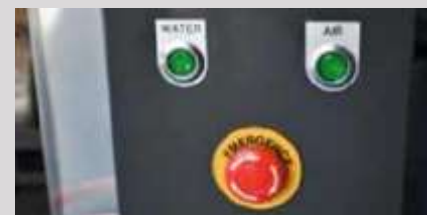
Emergency stop button
